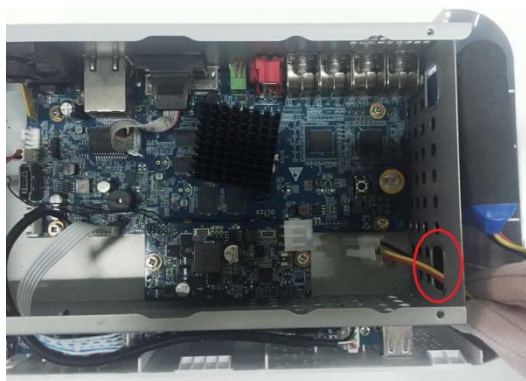
Figure 2-6 Pull battery cable through hole
