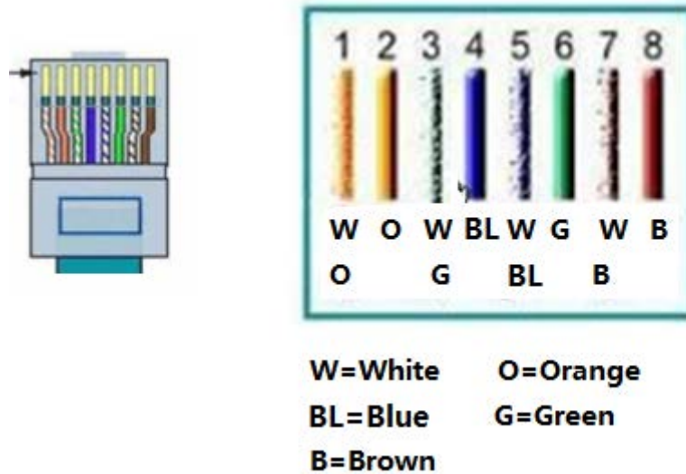
Appendix Figure 8-1 RJ-45 definition
